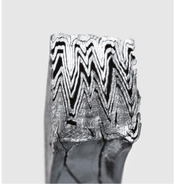
↑ Die-formed packing ring made of SIGRAFLEX tapes for use in stuffing boxes.
